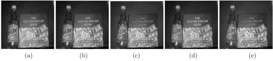
Fig. 2. Fusion Results of Multifocus Book Image (a),(b) Source Images (c) Proposed Method (d) Li's Method [4] (e) DWT based method [1]
