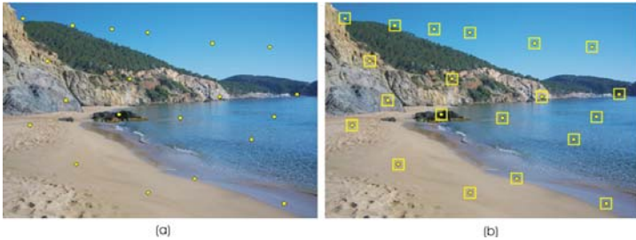
Fig. 2. (a) For sub-image description 300 image pixels are automatically and uniformly selected at random. (b) For automatically image segmentation around each of the 300 pixels a square window of M \times N is opened. In this figure only 20 points are shown as an example.
