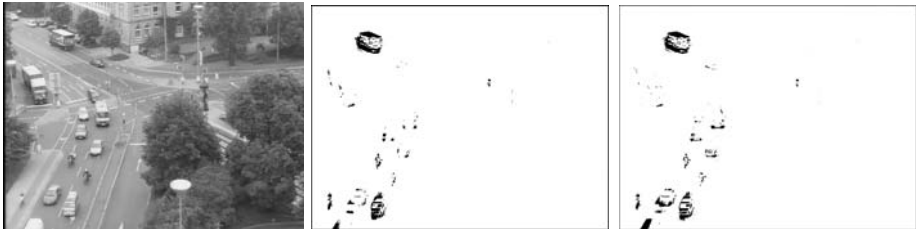
Fig. 2. (a) Original sequence, (b) Original algorithm results, (c) Change-Driven modified algorithm with 80,000 pixels (20%)
