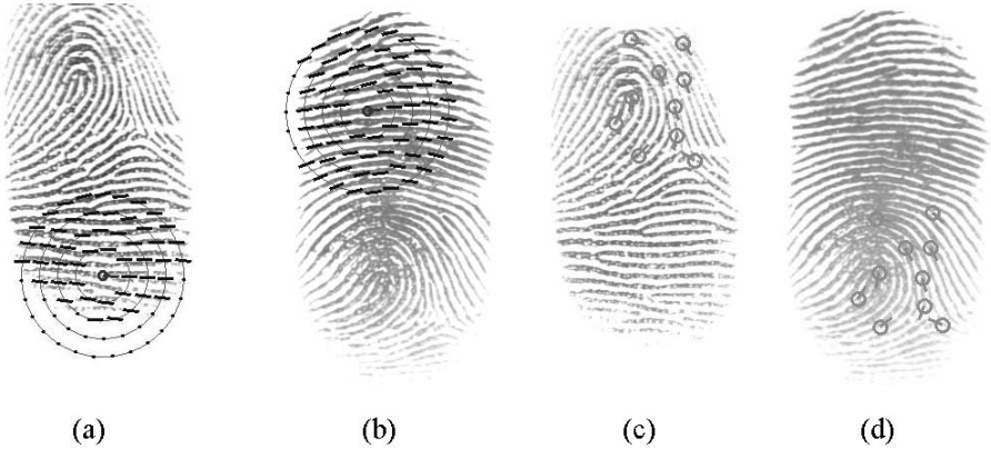
Fig. 2. The matching minutiae found by TK in fingerprints (a) 11_1 and (b) 11_3 from DB1_A in FVC2004. This is an example of a false matching minutiae pair that maximizes the possibility value in two fingerprints from the same finger. Images (c) and (d) show the good behavior of the modified TK algorithm while the original TK fails.
