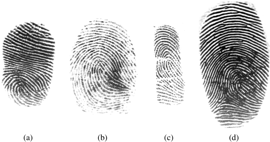
Fig. 3. These are two pairs of false not matching fingerprints from DB1_A using MTK. Fingerprints (a) 17_3 and (b) 17_6 are false not matching due to the high distortion on fingerprint (a). Fingerprints (c) 10_2 and (d) 10_4 are false not matching due to the small area of fingerprint (c).
