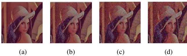
Fig. 3. (a) Original image, that is figure 2(a); (b) Image (a) with salt &pepper noise; (c) Image (a) with Gaussian noise; (d) Image (a) with both Gaussian noise and salt &pepper noise
