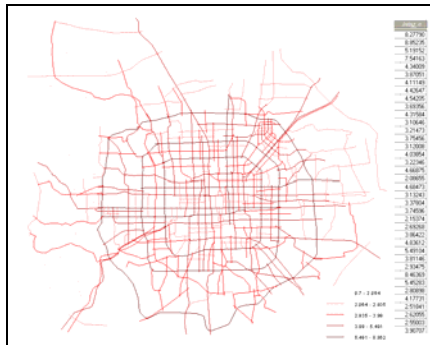
Fig. 3. Road axis graph and its attribute table in Beijing after integration improvement
