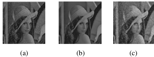
Fig. 5. (a) The image both Gaussian noise and salt & pepper noise. It's the grave-level of figure 3(d); (b) Image (a) after denoising with wavelet transform; (c) Image figure 4(b) after denoising with median filter.
