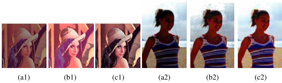
Fig. 11. (a1), (a2) is Original image. (b1), (b2) is the result image after histogram equalization directly on I componet. (c1), (c2) is the result with our algorithm.
