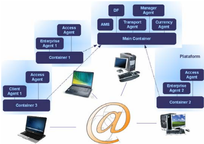
Fig. 5. The platform distributed architecture
