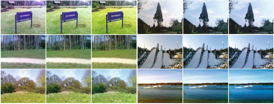
Fig. 3. Samples of the final white balanced images in sRGB . The columns from left to right illustrate the white point estimation using gray-world, refined gray-world, and ground truth, respectively.
