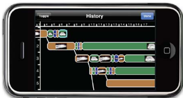
Fig. 5. History Browser Interface: horizontal axis represents the absolute time-scale of the synchronized videos; vertical axis represents branches showing user interaction
