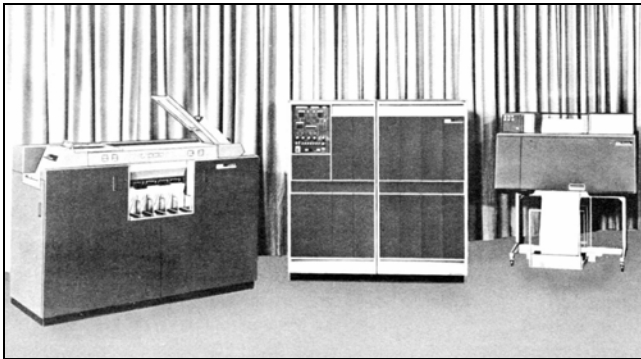
Fig. 5. The IBM 1401 configuration that Skýrr installed in the year 1964 consisting of card reader/punch, the central unit, and a line printer
