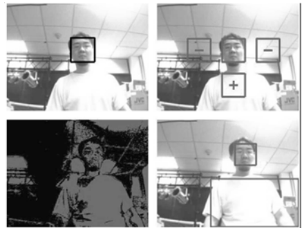
Fig. 5. Training and testing of the shirt-classifying algorithm. Top-left: face-detection; top-right: positive and negative sampling of the shirt; bottom-left: Boolean mapping of shirt colors onto image; bottom-right: shirt detection.
