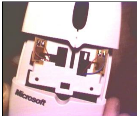
Fig. 1. Computer mouse with pressure sensors on buttons
