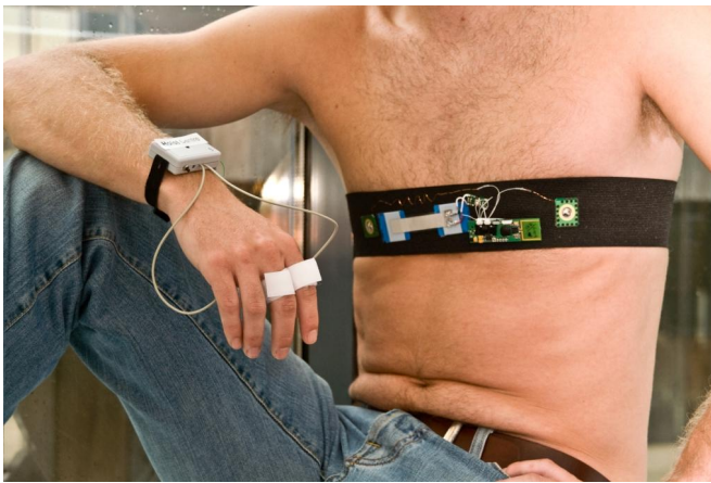
Fig. 1. Integrated body area network for ambulatory monitoring of physiological responses from the Autonomic Nervous System
