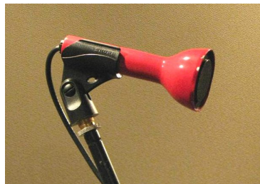
Fig. 3. The Soundbeam ultrasonic sensor
