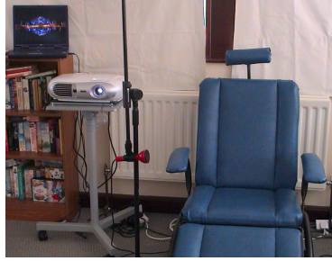
Fig. 2. The Soundchair, Soundbeam sensor, projector and computer
