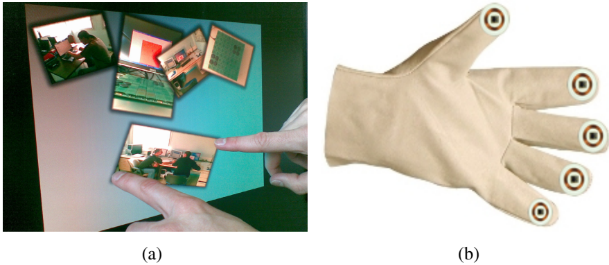
Fig. 3. An example of tactile display (a) and inclusion of RFID tags on a glove (b)
