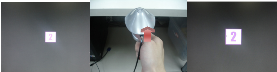
Fig. 8. The left one is the former image of a cube, when the user pushes the camera forward, the cube's size will increase as is shown in the right picture
