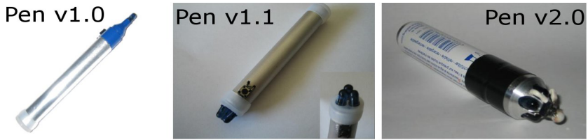
Fig. 2. Three versions of an IR LED Pencil for the operation of the Wii electronic Whiteboard. Pen v1.0 and pen v1.1 are using LED and a switch. Pen v2.0 is using the integrated switch on the tip of the pencil.
