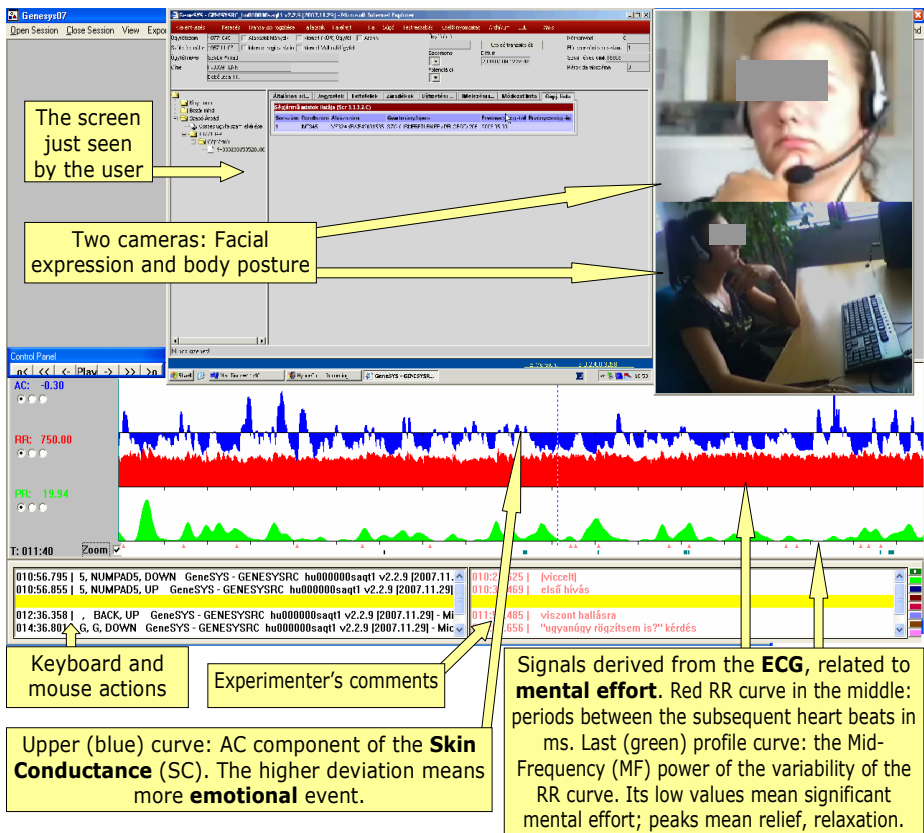
Fig. 3. The INTERFACE Viewer screen with a record of the empirical test of the Genesys software. As it can clearly be seen, currently the user makes significant mental effort – it is shown by the facial expression and gesture, and the low value of the last green profile curve of the Mid-Frequency (MF) power of the Heart Rate Variability (HRV) at the cross-hair.
