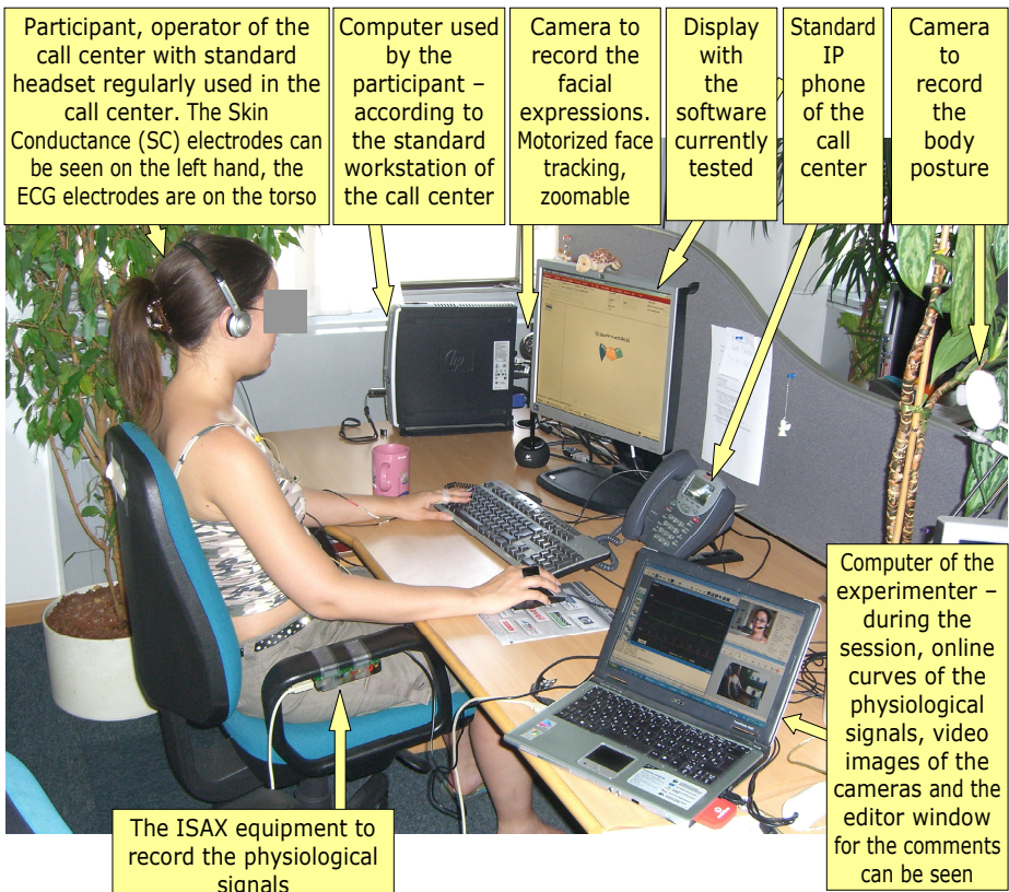
Fig. 2. The experimental arrangement applied during the sessions of the INTERFACE usability testing installed on a standard workstation of the call center
