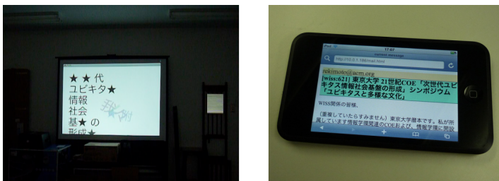
Fig. 5. Actual operation example. The picture on the left shows a peripheral display of Richbiff. On the right is a Web browser showing a current e-mail message reported by the peripheral display.
