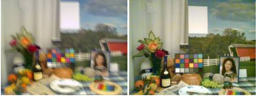
Fig. 3. Two example images from the testing in 100 lux illumination. The exposure times in left and right are 230 and 29 ms, respectively. This causes motion blur in left and noise in right side image. The subjective brightness of the images is adjusted to the same level by using appropriate gain factors. The three laser spots are clearly visible in both images.
