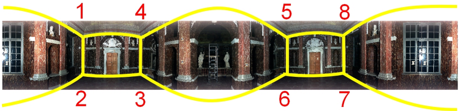
Fig. 3. Interactive user input (selection of eight points, or six geometric primitives). The shown arcs only illustrate how straight segments are curved in a cylindrical projection; they are not required for interactive input.
