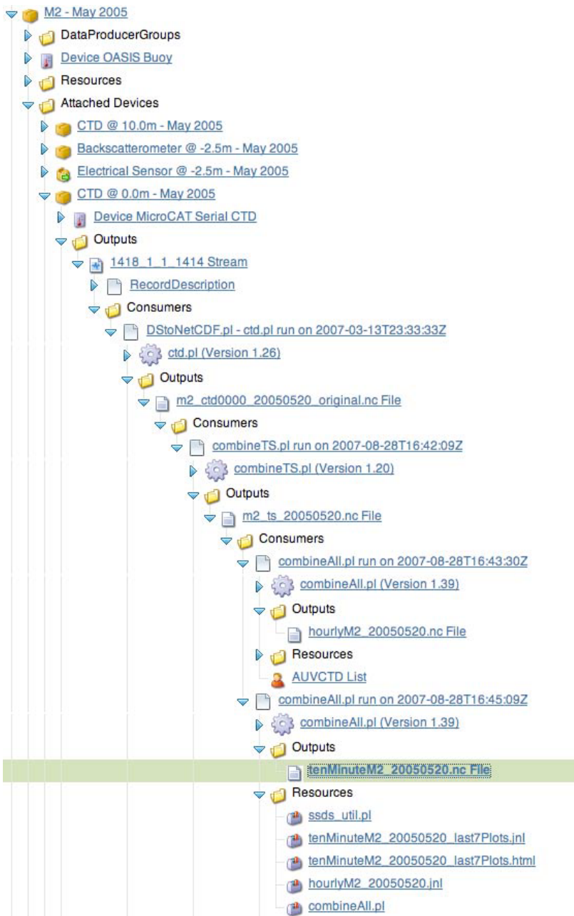
Fig. 6. Web application display of OASIS Buoy deployment’s CTD Device output and the chain of ProcessRuns and Outputs that finally combine data from the other instruments into a gridded tenMinute NetCDF data set the. Ancillary output from the combineAll.pl ProcessRun are recorded as Resources.
