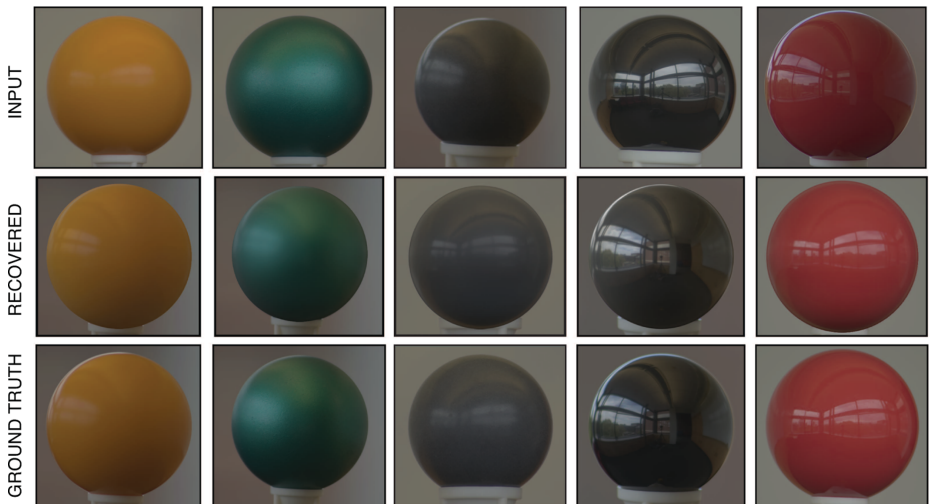
Fig. 8. Results using captured data. A BRDF is estimated from a single input image ( top ) under a known environment. This recovered BRDF is used to render a synthetic image for novel view within the same environment ( middle ). An actual image for the same novel position is shown for comparison ( bottom ). Despite the existence of non-idealities such as surface mesostructure and spatial inhomogeneity, plausible BRDFs are recovered.
