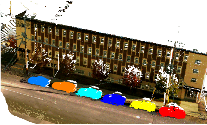
Fig. 1. Cars detection results from real LIDAR data. Cars have false colors.
