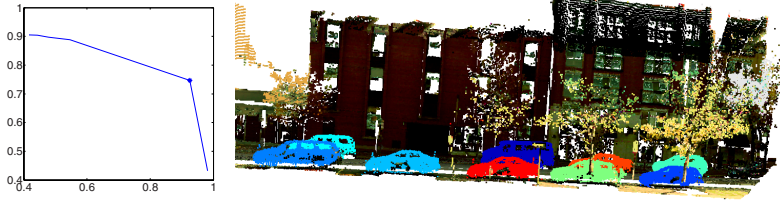
Fig. 6. Left: The precision-recall curve for car detection on 200 million points containing 1221 cars. (Precision is the x -axis and recall the y -axis.) Right: Screenshot of detected cars. Cars are in random colors and the background in original colors.
