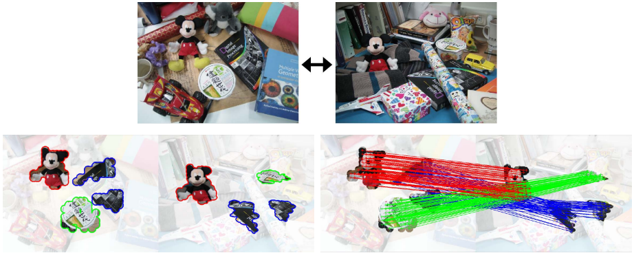
Fig. 1. Result of co-recognition on our dataset Mickey's . Given an image pair, co-recognition detects all Maximal Common Saliencies without any supervision or prior knowledge. Each color represents each identity of the MCS, which means an object in this case. Note that the book (blue) is separated by occlusion but identified as one object. See the text for details.
