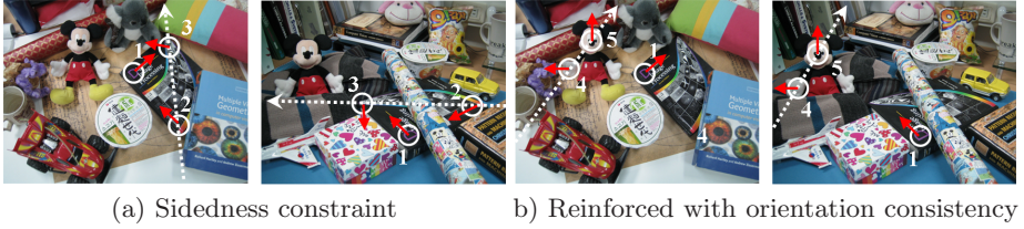
Fig. 3. (a) 1 should be on the same side of the directed line from 2 to 3 in both images. (b) 4,5 and 1 satisfies sidedness constraint, while it does not lies on the same object. We can filter out this outlier triplet by checking if orientation(red arrow) changes in the triplet are mutually consistent.
