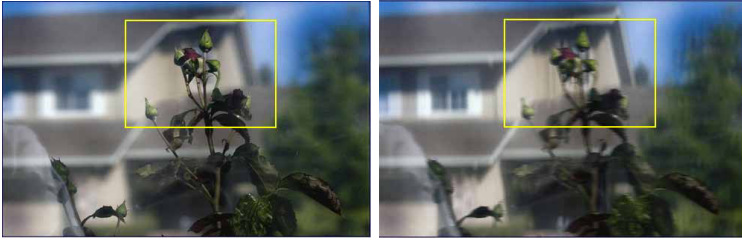
Fig. 8. Refocused images from our mosquito-net-based camera
