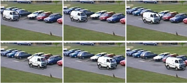
Fig. 5. Results on PETS 2001 sequence with temporal constraints. Motion layer boundaries are superimposed on the images. The windshield of the van is always classified as foreground. \lambda_0 = 0 , \lambda_1 = 30 , \lambda_2 = 17 and \lambda_3 = 15 .
