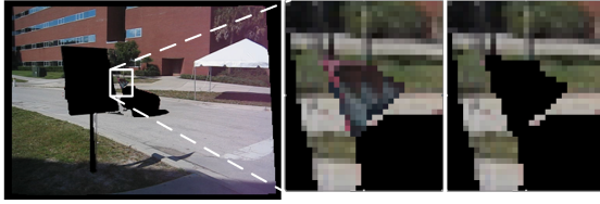
Fig. 9. Mosaic of the background. From left to right: obtained mosaic after first pass, detail of the white square that wrongly includes some parts of the car, misclassification removal by the user. In black, remaining holes in the mosaic: these regions are never visible in the processed interval.
