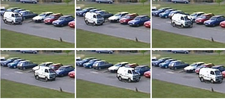
Fig. 4. Results on PETS 2001 sequence without temporal constraints. Motion layer boundaries are superimposed on the images. Note the temporal inconsistencies on the windshield of the van, due to its transparency. \lambda_0 = 0 , \lambda_1 = 30 , \lambda_2 = 17 and \lambda_3 = 0 .
