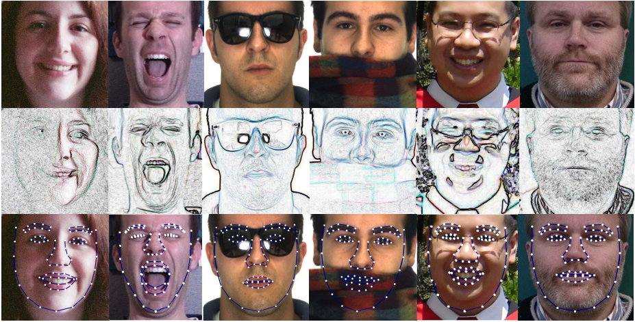
Fig. 1. Real-world face images could be extremely noisy in the eyes of computers. As shown in the gradient feature maps (second row), face topologies could be significantly corrupted due to various kinds of factors. However, our model can still recover sufficient shape details from such noisy observations while using a simple gradient-based landmark detector. The third row shows our alignment results.
