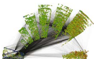
Fig. 16. Luxembourg roads, decomposed by reach, color indicates betweenness
