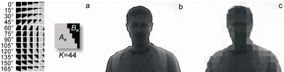
Fig. 2. a. The 60 kernels and the 44 th kernel in magnification. b. The Y component of the original image. c. The orientation map OM of image b.
