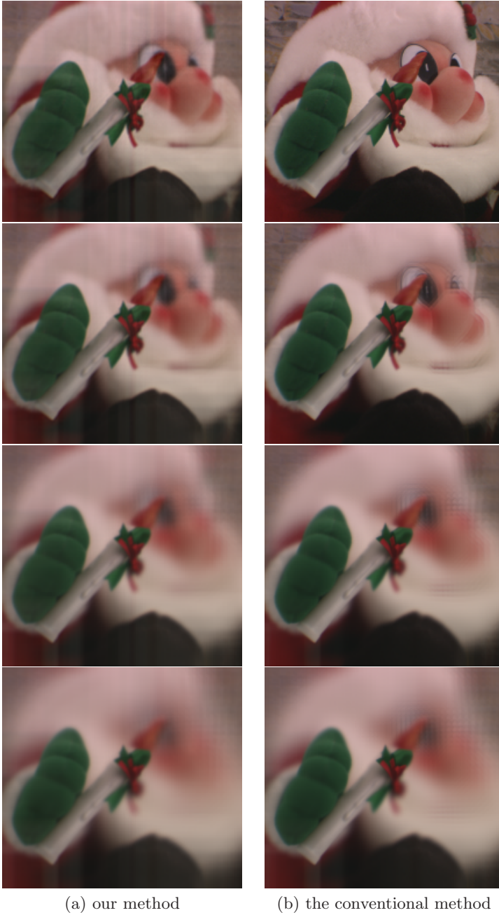
Fig. 6. Results for real multiview images when the aperture radius R is varied at 0.5, 1.0, 2.0 and 3.0 times of the distance between cameras. The focal depth was fixed at 590.
