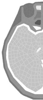
Fig. 1. FEM brain structure showing different materials: skin, bone of the cranium, brain's fluid and brain tissue. It is a horizontal slice at eye level. For the purposes of symmetry is a semi-piece.
