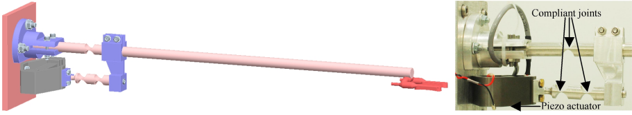
Fig. 4. The current prototype of the active stabilizer. On the left, a CAD global view and on the right the detail of the closed-loop mechanism on the current prototype.
