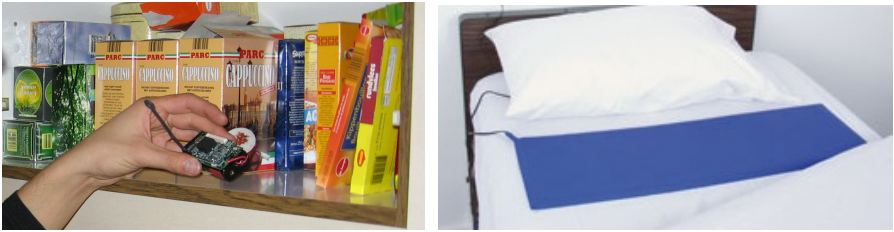
Fig. 7. Placing a wireless mote with a photo sensor in a cupboard(left), an illustration of a pressure pad used for bed-activity detection (right)
