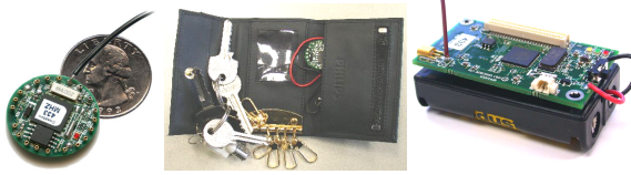
Fig. 6. From left to right: mica2dot mote, key fold with mica2dot, and mica2 mote
