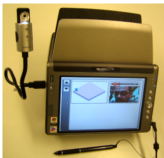
Fig. 5. The storytelling application in a Tablet PC with a webcam attached to it
