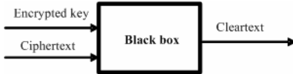
Fig. 1. Black-box model with inputs of encrypted key and ciphertext and it outputs cleartext
