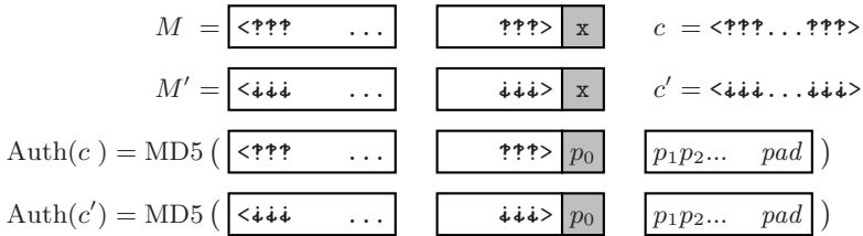
Fig. 1. APOP password recovery through MD5 collisions
