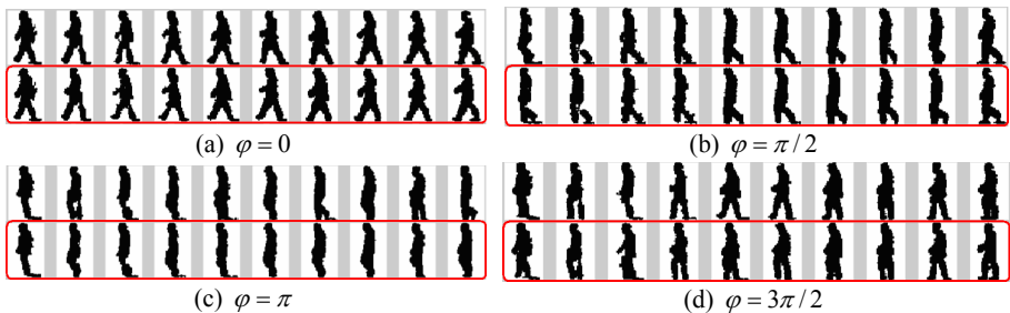
Fig. 3. Examples of CPFs on 4 phases from one of our test sequences. For each phase, the first row shows CPFs coming from the fixed period detection, while the second row enclosed by rounded rectangle corresponds to CPFs coming from the adaptive cycle detection.
