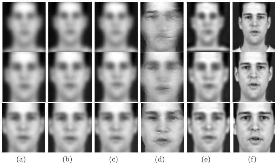
Fig. 2. Comparison between enhanced images. First row 90 \times 72 , second row 120 \times 96 , third row 180 \times 144 . (a) bilinear interpolation, (b) cubic spline interpolation, (c) Schultz et al., (d) Baker et al., (e) Lin et al., (f) ground-truth.
