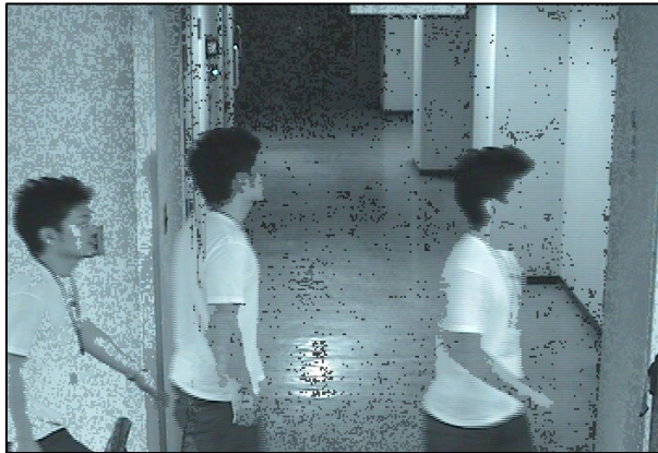
Fig. 6. Gathered image of time period that contains lighting. Information of lighting can be obtained, although there is a part in which the person disappears, depending on their color.
