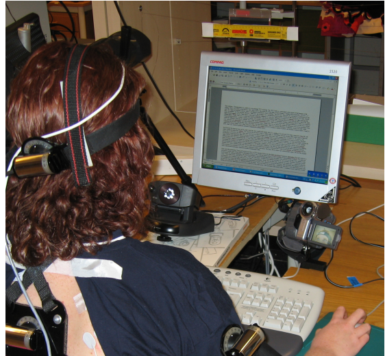
Fig. 2. The video camera used to record eye blinking is seen below and to the left of the VDU-screen
