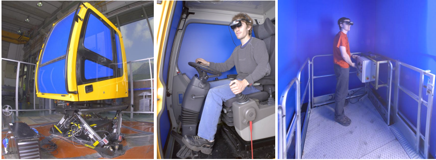
Fig. 1. Hardware setup: Exterior (left) and interior view (middle) of the real excavator cabin used for excavator and dumper simulation. The blue-box used for mast climb platform and lift simulation, also mounted on the motion platform (right).
