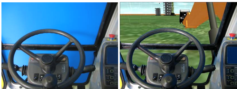
Fig. 5. Chroma-key: Original image (left) and final image, after blue screen matting (right)
