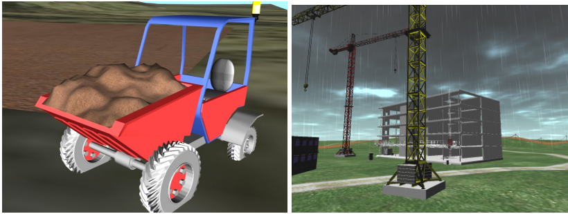
Fig. 2. Virtual reality. The virtual scene has been implemented using OpenSG as the graphics engine and ODE for the physical behavior. GPU shaders have been used to render the weather conditions (rain, fog, clouds) and the soil to enhance the realism of the scene.
