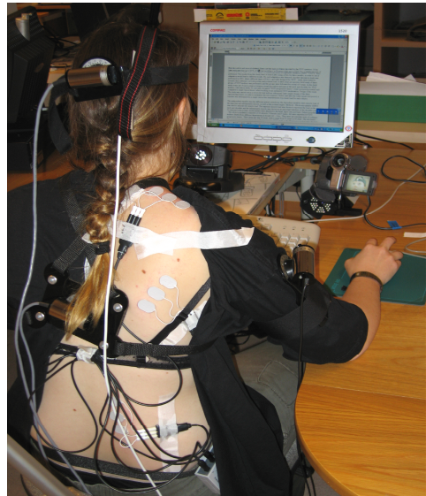
Fig. 1. Electrodes and angles sensor used by the Physiometer
