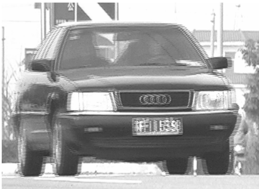
Fig. 1. An example of interlaced effect on moving object
