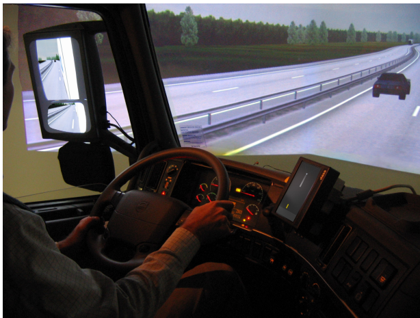
Fig. 8. LRM display mounted in the truck dashboard
