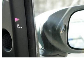
Fig. 5. HMI solution addressing the LCW application for car (a-pillar, red)
