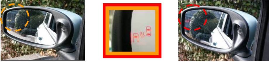
Fig. 3. HMI solution (side-mirror led) for the lateral area of the vehicle addressing LCA and the lateral functionality of the LRM for cars applications
