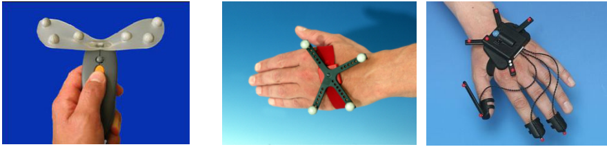
Fig. 3. Interaction devices “FHG-IAO Hornet” (left), ART hand target (middle) and ART finger tracking (right)
