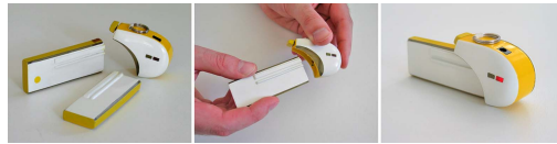
Fig. 1. Activation of the Personal.Aura artefact by connecting an ID Stick to the Reader Module
