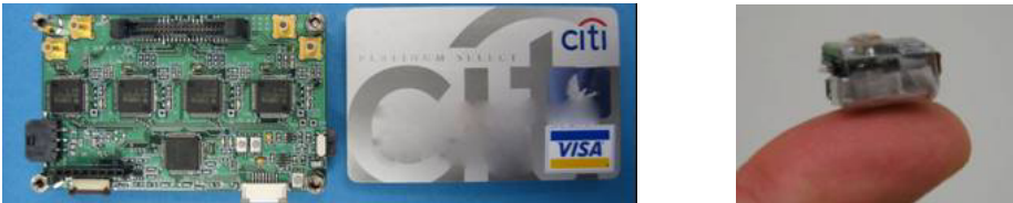
Fig. 5. (left) Prototype data acquisition board with credit card for scale. (right) Prototype miniature wireless transmitter.
