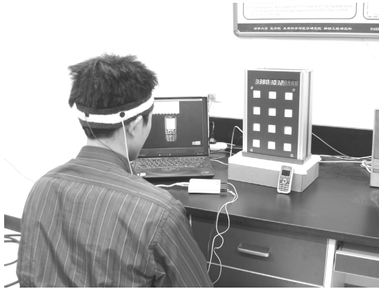
Fig. 4. The brain controlled HCI box in the operation of dialing a cell phone number
