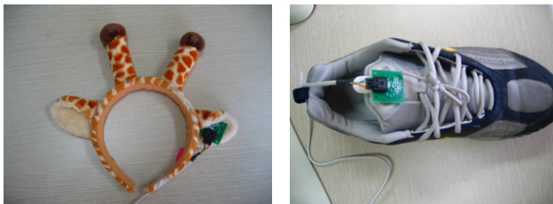
Fig. 3. Acceleration sensor attached hair band and shoe
