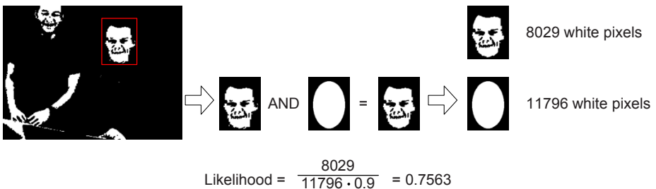
Fig. 2. An example of how the skin color likelihood is calculated for \beta = 0.9
